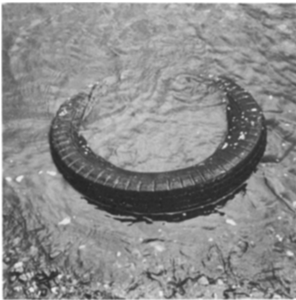
Figure 1 General view of tyre during recovery after 42 yr immersion in sea-water.
