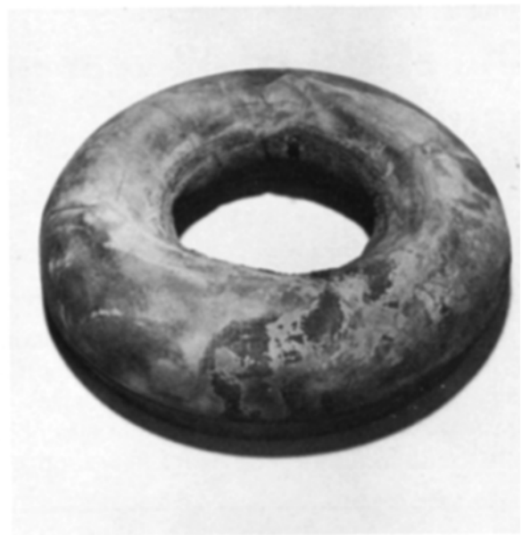
Figure 3 General view of truck inner tube after 42 yr immersion in sea-water — shown inflated in the laboratory.
